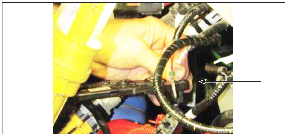
Figure 5 - Crimp the Assemblies
