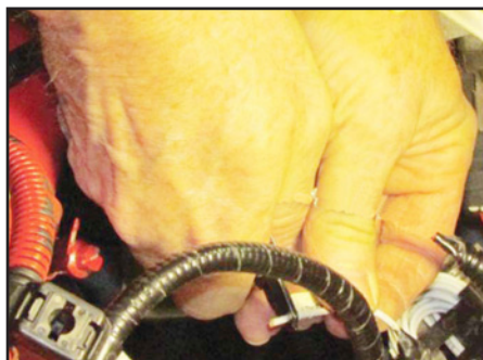
Figure 3 - Cut and Bare the Wires
