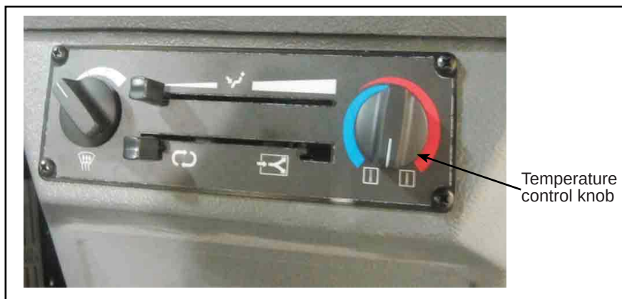
Figure 1 - Operator's Heater Control Panel
