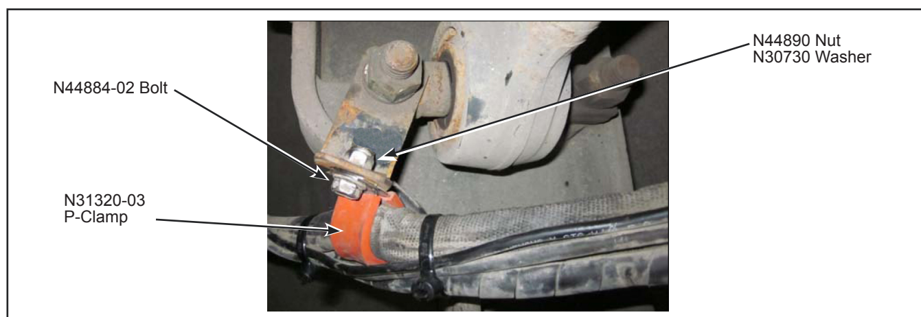
Figure 8 - L Support and P-Clamp Installation
