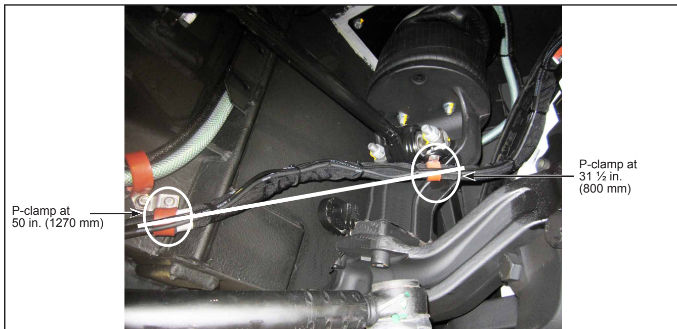
Figure 9 - P-Clamp Alignment at the 31½ in. (800 mm) and 50 in. (1270 mm) Positions
