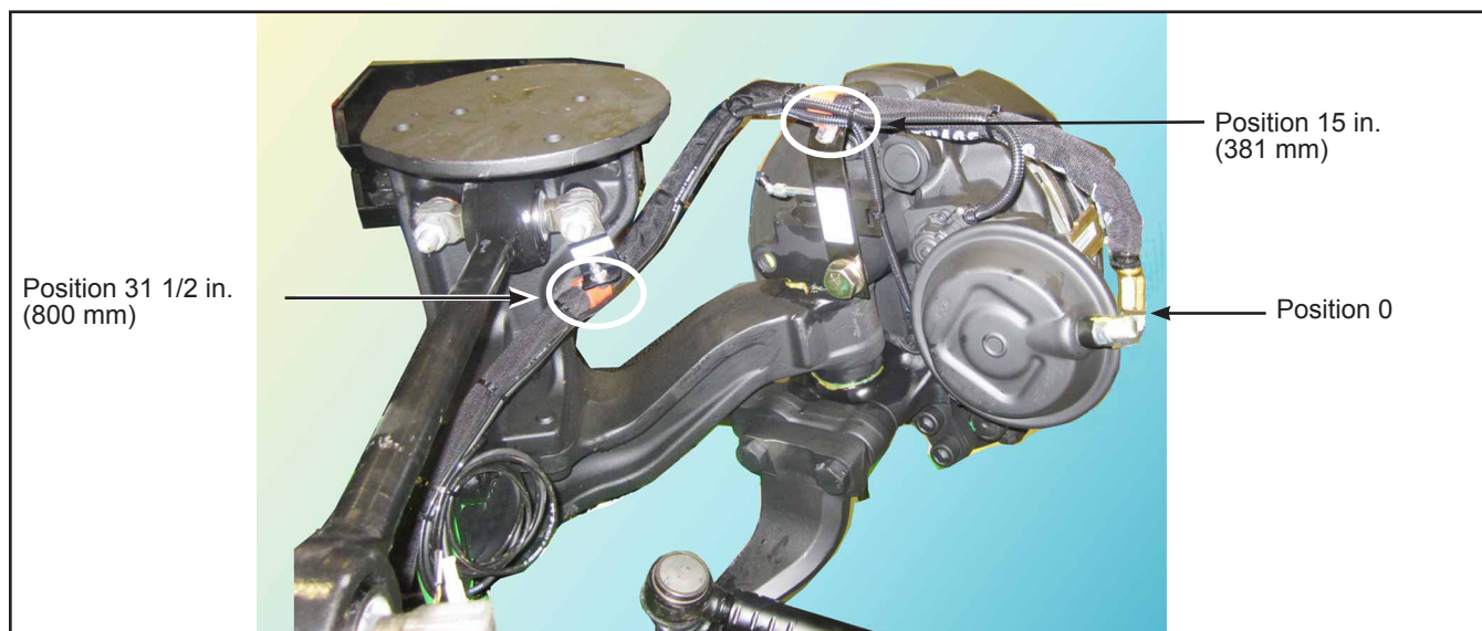
Figure 3 - P-Clamp Location on Hose
