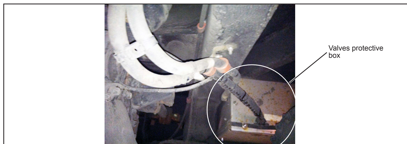
Figure 24 - Brake Valves Protective Box
