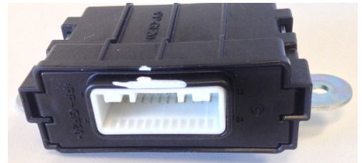
The Smart Connector communicates via LIN communication to control the mirrors and is equipped with a new semiconductor component called the Mirror IC. The mirror control logic is located in the IC CPU.
