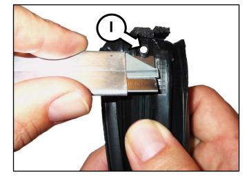
10. Carefully install the glass run channel(J) around the window frame.
