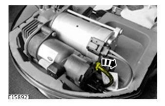
**8.** Remove the exhaust valve end cap and spring.
