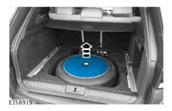
3. Remove spare wheel fixing.
