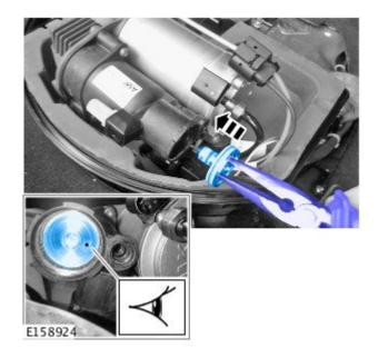
11. NOTE: Make sure the spring is pushing behind the valve.
