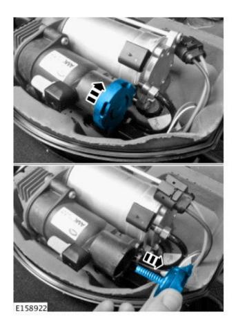
**9.** Pull out the exhaust valve from the housing.
