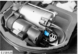
13. Install the 8mm outlet pipe into the adaptor.
