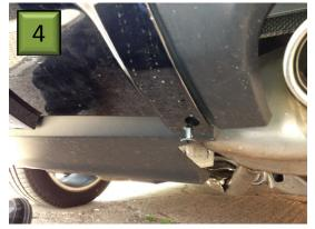
1/ Please ensure the fixings are set in this direction and free ready for installation.
