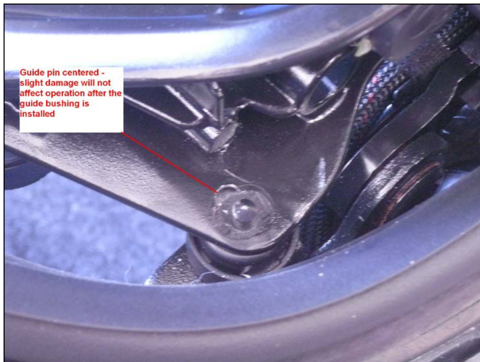
Figure 4: Guide pin centered after adjustment and before installation of new guide bushing.
