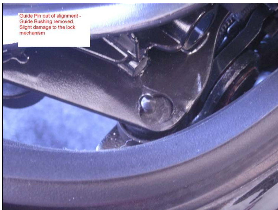
Figure 2: Guide pin out of alignment (shown with bushing removed)
