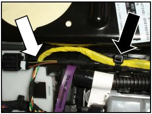
For seats without holder (previous illustration), it may be necessary to utilize a zip tie (shop supply) as shown –black arrow-, and/or route harness under existing wiring as shown –white arrow-
