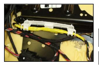
If Yazaki connector (previous picture) has been removed and seat wiring harness repaired as pictured, Work Complete for that seat, reposition seat to customer original setting(s)
