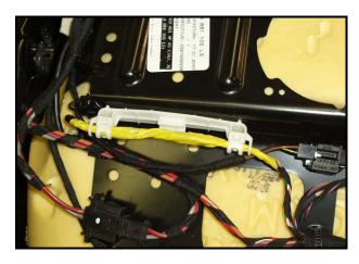
Wrap repaired area of harness with yellow tape and re-secure into holder (if equipped) as shown
