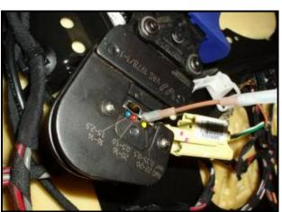
Insert each stripped wire into butt connector of corresponding repair wire and crimp butt connector as shown using –VAS 1978/1-2crimping tool pliers with –VAS 1978/1-1- crimp head using 0.35mm-0.5mm (yellow dot) setting
