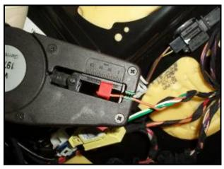
Set –VAS 1978/3- wire stripper to 6mm and strip insulation from the end of each wire as shown
