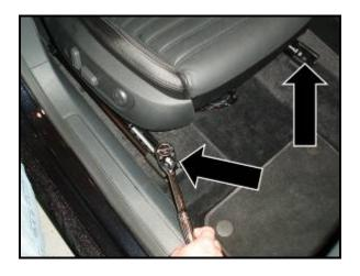
Tip: Centering pins on tunnel side must be located in corresponding holes in vehicle floor
