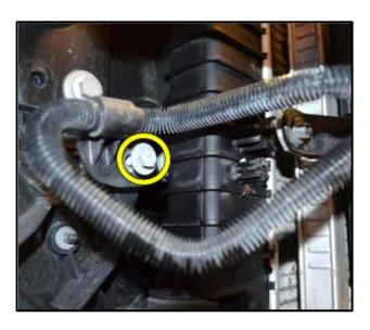
Loosen the mounting bolt for the power steering fluid cooler <circle>.
