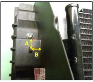
WARNING! Perform the next two steps with the passenger side radiator shroud removed from the vehicle. This will prevent damage to the radiator. Damage to the radiator will not be covered under this action.
