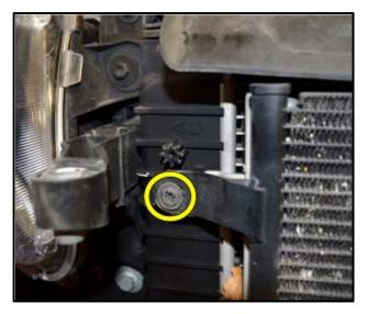
Remove the upper and lower mounting screws from the passenger side of the charge air cooler <circle> and discard them (upper screw shown).
