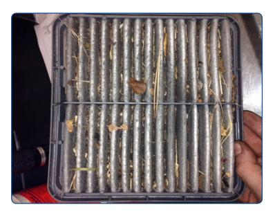
When performing diagnostics for engine-related problems, don't forget the simple items which can easily be overlooked. Recently, a vehicle with only 27,420 miles was brought in to a dealership for misfire codes P0301, 302, 303, 304. The air filter was almost completely clogged (see photo to the left). Even when a vehicle has not reached a point where maintenance items would be inspected or replaced (ex: air filter at 30K), they should still be checked as part of the diagnostic procedure.
