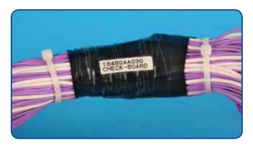
The CHECK-BOARD is a series circuit harness with parallel circuit connectors which fits in between the ECM and the ECM harness connectors. When installing, always connect the weatherproof connectors to the ECM.
