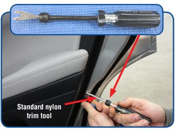
Use a standard trim tool to widen the gap between the trim panel & the door panel near the clip location & then insert a slotted trim tool into place at the designated clip to carefully disengage the clip by twisting the tool.
