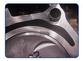
The deck surface of some remanufactured short blocks will sometimes exhibit a difference in finish texture, as shown in the picture.
