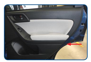
After removing the panel gusset piece & mount screws, remove the clip designated with an arrow above before releasing any other panel mount clips
