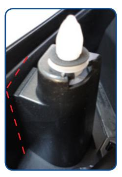
Other panel clips are much more supported in a variety of designs and we have encountered no damage to the supports at any other clip locations during panel removal
