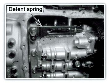
**15.** Remove 8 bolts in the order shown and remove the valve body.
