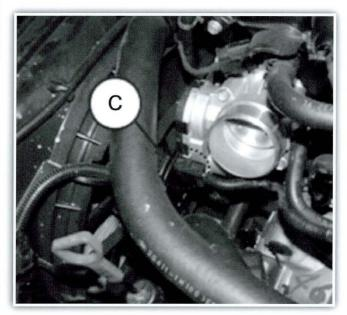
**3.** Remove the 4 ETC throttle body mounting bolts and then pull out the ETC throttle body away from the intake manifold.
