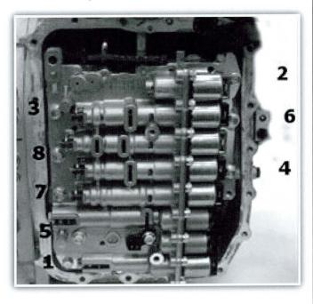
**16.** Use a screwdriver to depress the locking tab and pull outward on the connector to the input and output speed sensor.
