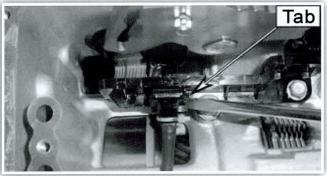
**17.** Remove two bolts that secure the valve body harness to the case.
