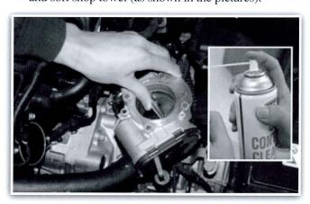
NOTE: Do not use excessive force to open the throttle valve. Be careful not to scratch the throttle valve and bore area during cleaning.
