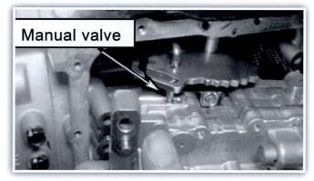
**20.** Install the valve body bolts and torque the bolts to specification in the order shown.
