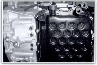
23. Remove the transaxle fill plug.
