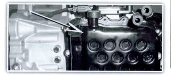
**11.** Use a small screwdriver to pry the connector from the oil temperature sensor.
