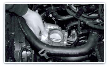
**4.** Spray a carbon cleaner or throttle body cleaning solution on the throttle valve and bore areas where deposits have accumulated. Wipe off the deposits with a clean and soft shop towel (as shown in the pictures).
