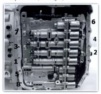
**21.** Reconnect the solenoid harness to the solenoids and oil temperature sensor.
