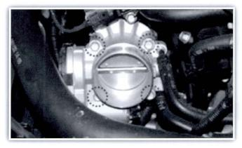
NOTE: Do not disconnect the coolant hose from the ETC throttle body. It is not necessary to remove the ETC throttle body completely from the vehicle for cleaning.
