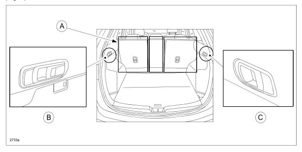
This concern may be caused by an incorrect seatback remote cable adjustment position. The current adjustment position may not provide enough tension for the cable to unlock the seatback latches.
