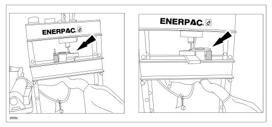
**NOTE:** Take care not to bend or damage the flange while pressing out the studs. Make sure both sides of the flange are supported as shown above.
