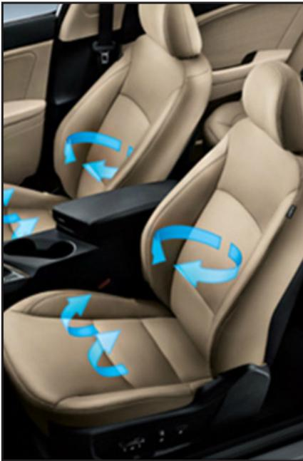
Some Sorento, Optima and Sportage vehicles are optionally equipped with ventilated front seats. These seats improve occupant comfort by drawing the ambient air of the vehicle interior through the seating surfaces.
