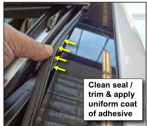
3. Carefully push the side trim seal back into the sunroof side trim and apply pressure for several seconds to ensure that it is properly positioned.
