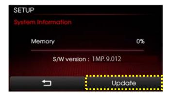
14. Check that "New Version" is correct for this Service Action (New version is 1.MP.9.013); if version is correct, then touch "Yes" button on screen.
