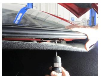
**Note:** Whenever you drill into a metal surface, the corrosion resistance of that panel is compromised. Treat the drilled holes with GM Supe Lube®, P/N 12371287 (in Canada, 10953437), to prevent corrosion.
