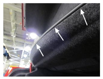
6. Once the push pins are installed, ensure the trim panel is properly tucked under the deck lid weatherstrip.
