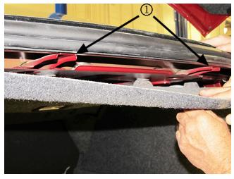
1. Pull the trunk trim panel downward to locate the two fore/aft metal braces (1) on the underside of the package shelf sheet metal.
