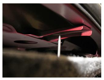
2. Line up the trim panel and brace for the new hole location and pierce a hole through the trim panel material and center punch the new hole location on the bracket. Repeat on the opposite side.
