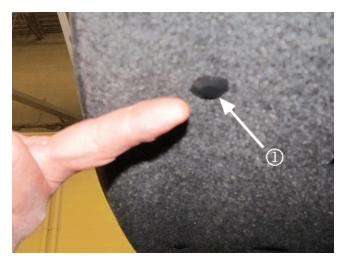
5. Reinstall the trim panel to the underside sheet metal and insert a GM push-pin, P/N 11562024 (1), through the trim panel and into the drille hole on each side.
