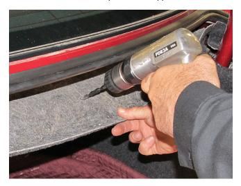
3. Using a ¼ in drill bit, drill a hole through the trim panel at the two locations that the trim panel was pierced.
