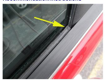
Using an appropriate tool, reposition the seal. Ensure it contacts the glass for the full length of the seal.
