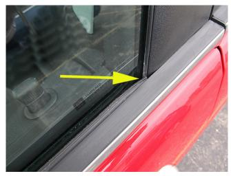
This condition may be caused by an out of position outer window belt sealing strip (side door window belt outer sealing strip).
