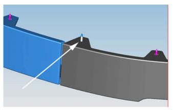
1. The two screws shown above are preinstalled at the plant and need to be removed from the wheelhouse liner prior to air deflector installation. Reinstall these screws first when installing the air deflector.
