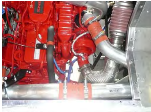
FIGURES 8 & 9. ISB DIESEL HYBRID ENGINE SHOWN
