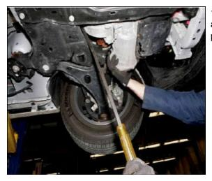
10. Using a long pry bar rock motor forward and block to support motor in the forward position.
