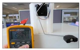
Is resistance measurement 290±0.5 ohms?
