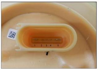
Measure the resistance between module pin terminals 2 and 3.
