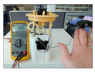
Raise the float arm up to the physical limit and measure the resistance between module pin terminals 2 and 3.
