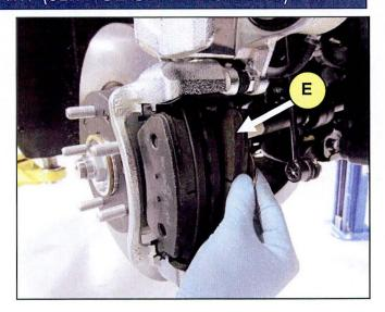
7. Remove the brake outer pad (F).
