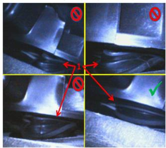
3. Reposition the seal (1) using a suitable hook tool or flat bladed tool as necessary.
