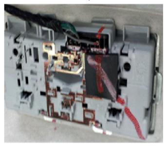
6. Inspect the back of the dome lamp to ensure the foam block is in place.
