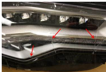
Figure 1. Cracks at bottom of headlight lens.
