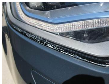
Figure 3. Stress fractures along lower edge of headlight lens.
