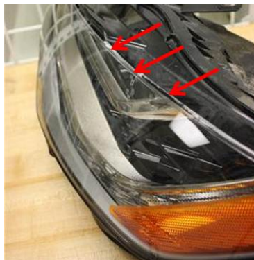
Figure 2. Cracks and separation along top edge of headlight lens.
