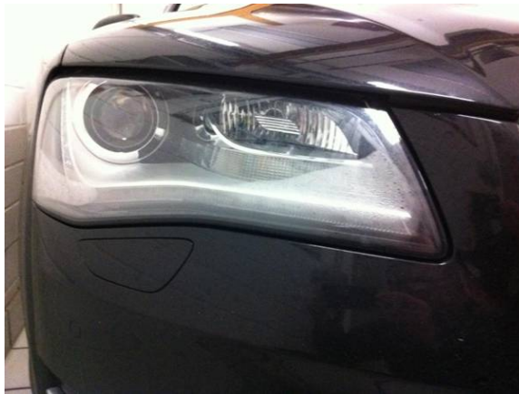
Figure 1. Example of a headlight with condensation inside the lens.
