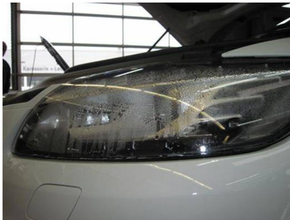
Figure 2. Example of a headlight with a leaking condition.
