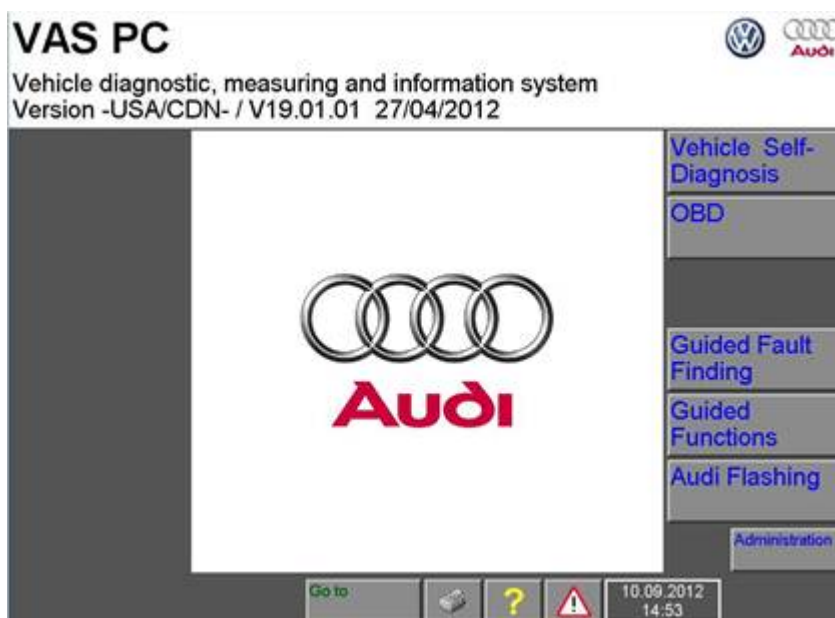
Figure 1. Select Vehicle self-diagnosis>>56 – Radio>>012 – Adaption.
