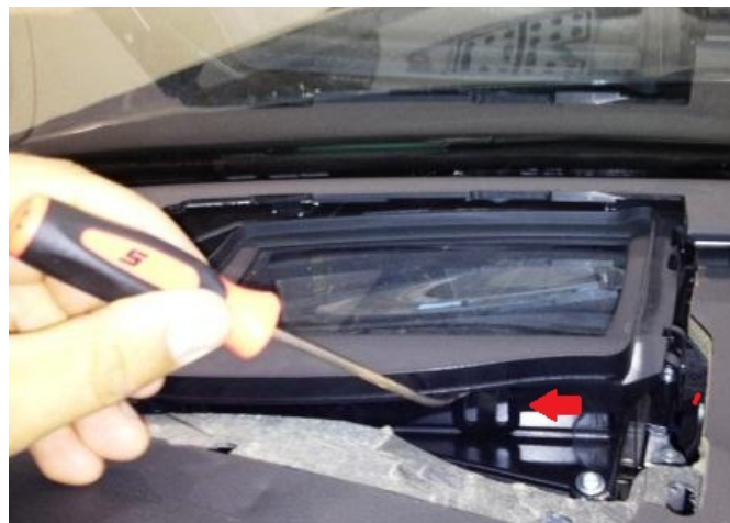
Figure 2. Carefully use a small angled pick tool to delicately disengage the six latches.
