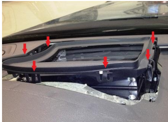
Figure 1. Six latches are shown with red arrows.
