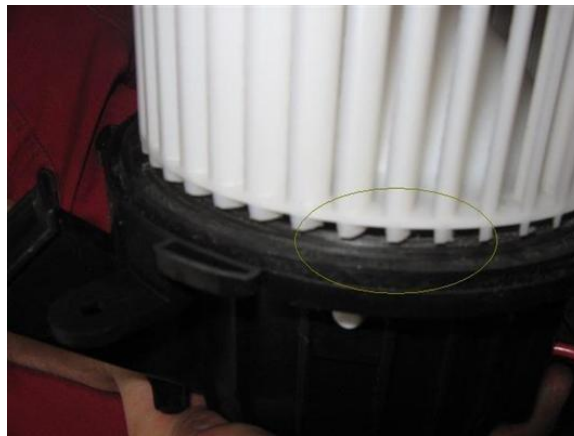
Figure 2. Interference of blower impeller to the lower housing.
