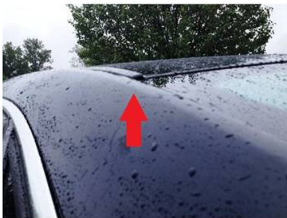
Figure 1. Roof joint strip loose.
