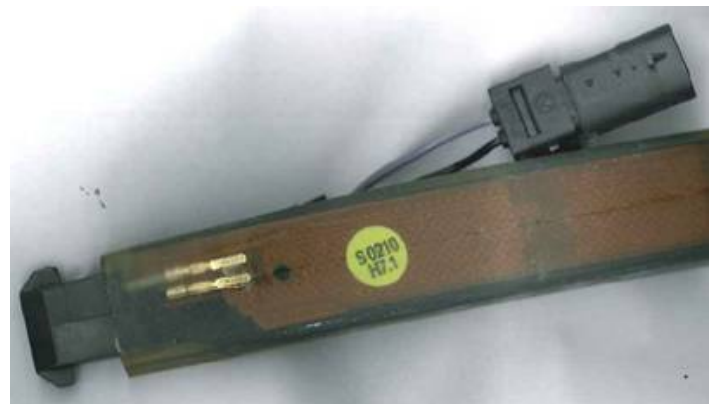
Figure 2. Door handle touch sensor version sticker.
