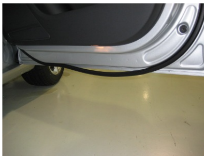
Figure 1. The outer door seal, partially detached.
