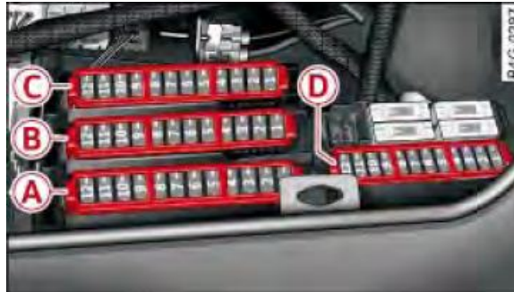
Figure 1. Fuse panel for A6/A7 vehicles.
