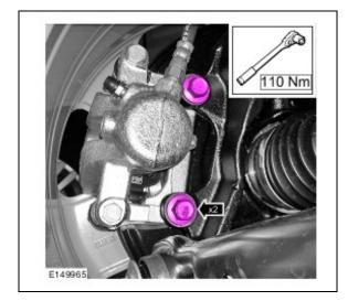
4. Repeat step 3 on the right-rear brake caliper.
