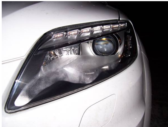
Figure 1. Moisture in headlamp.
