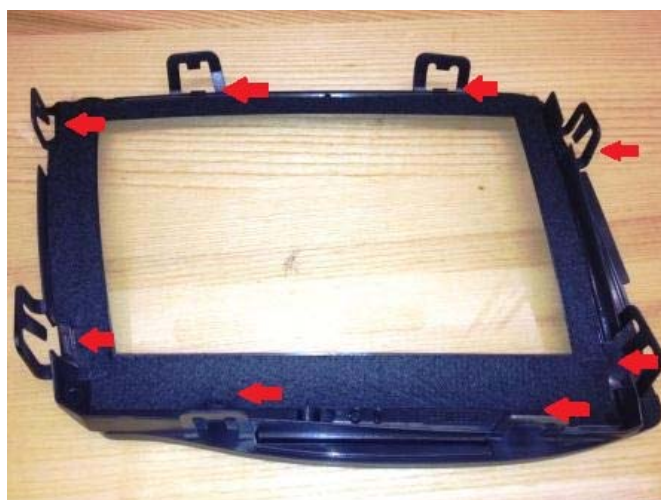
Figure 3. Eight positive standoffs that must not be covered by the felt tape are shown with red arrows.
