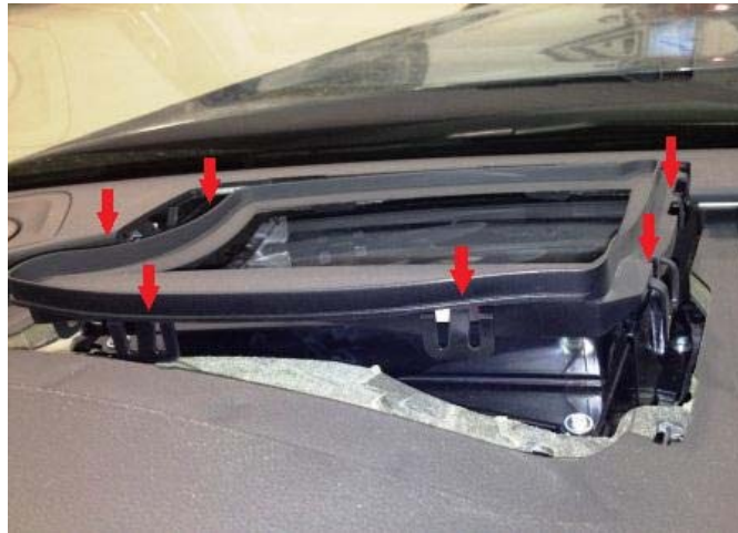
Figure 1. Six latches are shown with red arrows.
