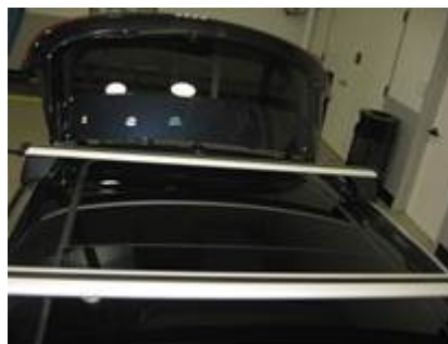
Figure 1. Roof carrier bars installed.
