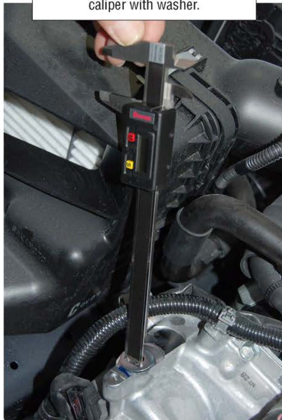
Measurement taken using digital caliper with washer.
