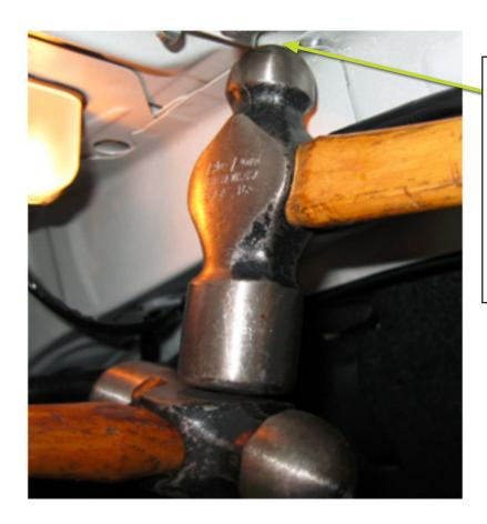
Photo shows positioning of tools used to close the gap between the plates.
