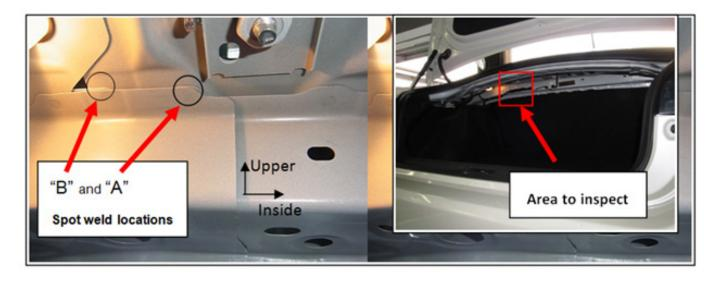
Using the tip of a flat-blade screwdriver, **CAREFULLY** separate the plates of the spot weld area "A" **ONLY** approximately 1/8" (3.5mm) as shown in the photo below. For spot weld area "B", only grease will be applied at this time.
