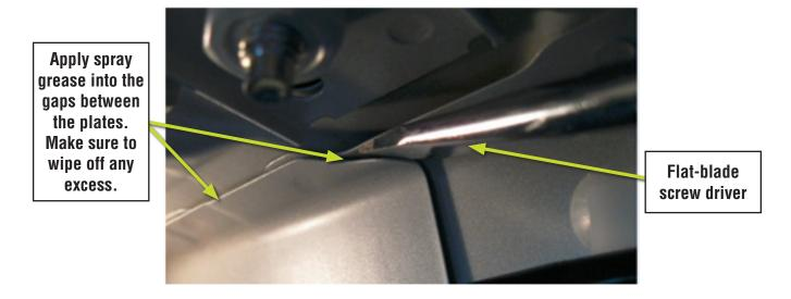
After spraying the grease into the gaps, use a suitable method to **CAREFULLY** reduce the gap between the lower and middle plates as shown in the photo on the next page. Take proper precaution to prevent damage to the paint.
