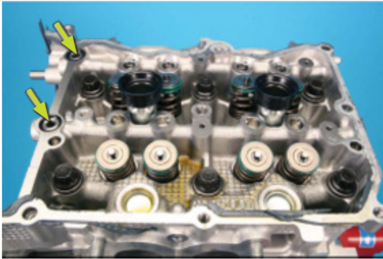
Cam carrier o-rings requiring replacement
