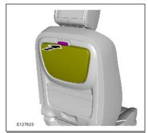
2.  $\triangle$  NOTE: If a washer is present behind the business tray latch, it must be installed in the same position on the new latch.
