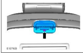
3. A NOTE: Make sure the latch is fully seated prior to installing and tightening the fixing.
