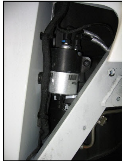
Figure 1. In-line fuel filter.
