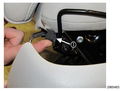
5.4. Install one of the seat cushion cover retainers (1) to the seat, pushing one leg through the slit in the fabric and the other over the seat frame, capturing the J-channel against the frame.
