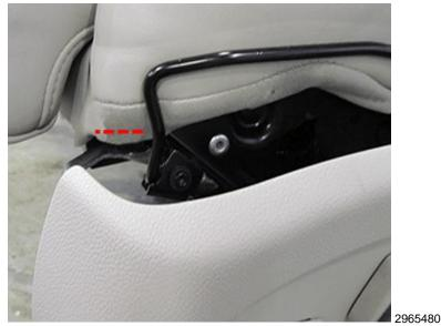
5.1. Fold the J-channel back under the cover fabric material, but do not attach to the frame. Note the location of the bottom edge of the channel through the material.
