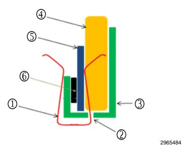
Note: A cross section of the clip installation is shown in the illustration above. Ensure the clip (1) is inserted through the slit (2) in the seat material (3), between the foam (4) and the seat frame (5), capturing the material and J-channel (6).
