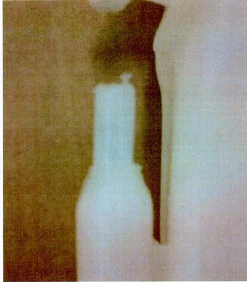
Fig. 2 Excessive Flash On Coolant Bottle Nipple - Hose Removed
