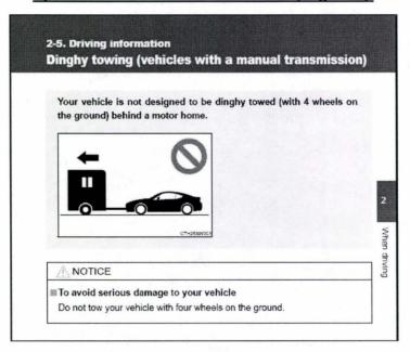
The Scion FRS is not designed to be dinghy towed with all four wheels on the ground behind a vehicle. Doing so may cause serious damage to the vehicle.
