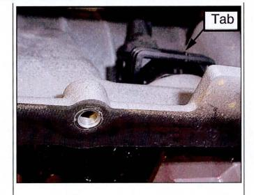
8. Use an 8mm or 5/16" hex socket and remove the drain plug and drain the ATF.
