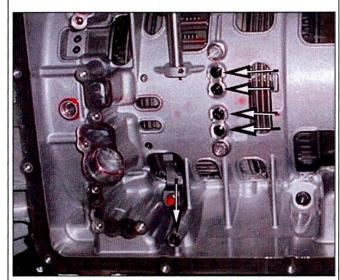
12. Align the manual valve to the shift lever and install the valve body.
