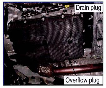
ATF TEMPERATURE = 122~140°F (50~60°C) SHIFT LEVER IN "P" AND ENGINE RUNNING
