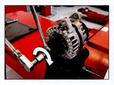
10. Remove the pulley from the alternator.
