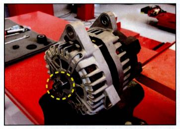
11. Install new OAP pulley onto the alternator shaft by hand. Using a wrench, pulley removal/installation tool and Torx® socket, secure the OAP pulley to the shaft by turning the socket <u>counter-clockwise</u>.
