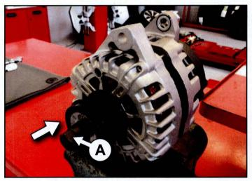
8. Insert the T-50 Torx<sup>®</sup> socket (B) through the pulley removal tool (A) and into the alternator shaft.
